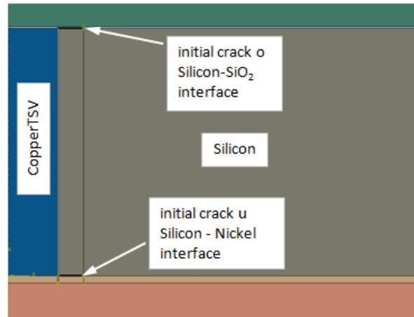
Fig. 3 Assumed initial delaminations at bi-material interfaces
