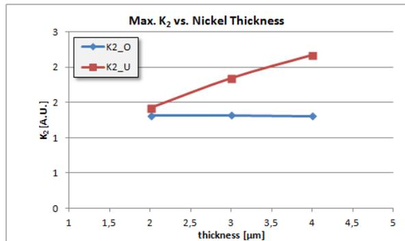
Fig. 8  $K_2$ -progress of both initial cracks vs. thickness of the Nickel layer
