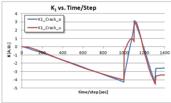
Fig. 5  $K_1$ - progress of both material initial cracks during thermal loading - see Fig. 4
