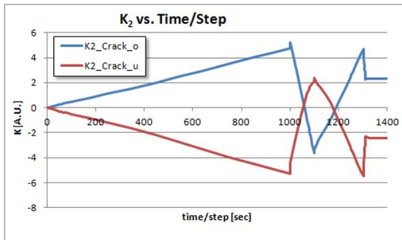
Fig. 6  $K_2$ -progress of both material initial cracks progress during thermal loading – see Fig. 4
