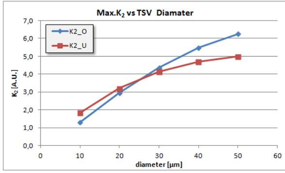
Fig. 10  $K_2$ -progress of both initial material interface cracks vs. TSV diameter
