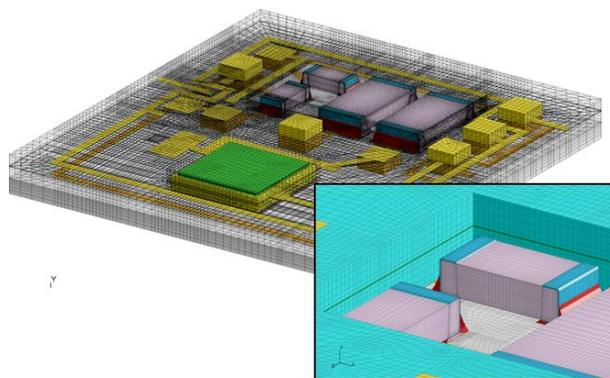
Fig. 1 2D/3D Wafer Level integration of a power module
