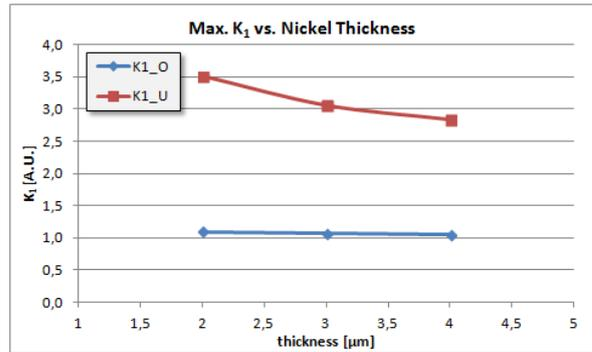
Fig. 7  $K_1$ - progress of both material initial cracks vs. thickness of the Nickel layer
