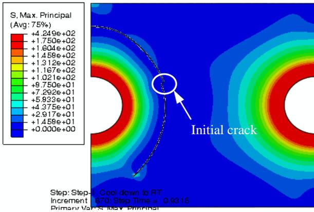
Fig. 14 Initial crack located between the 2 TSVs; cool down from stress free temperature 160 °C to RT
