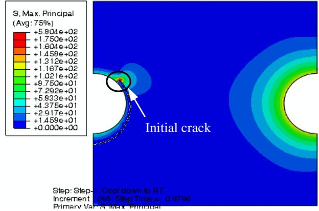
Fig. 11 Initial crack located at the side wall of one TSV; cool down from stress free temperature 160 °C to RT
