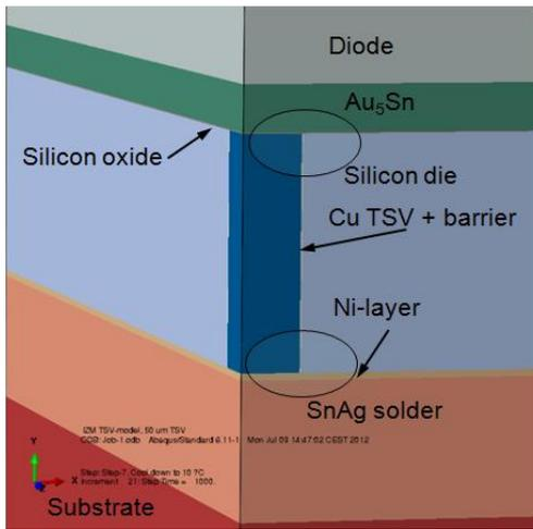
Fig. 2 Detail of the design of the LED-Package in the surrounding of a Copper-TSV
