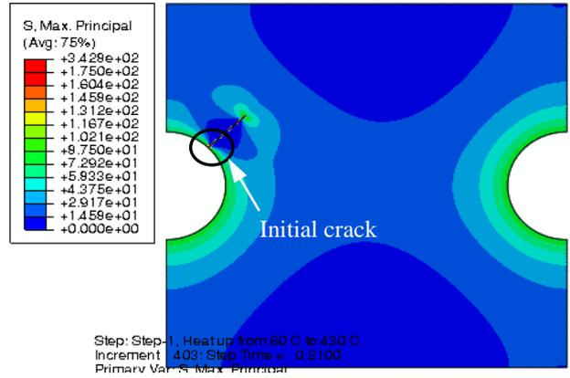
Fig. 12 Initial crack located at the side wall of one TSV; heat up from stress free temperature 60 °C to 430 °C
