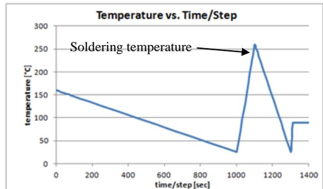
Fig. 4 Thermal loading during package handling
