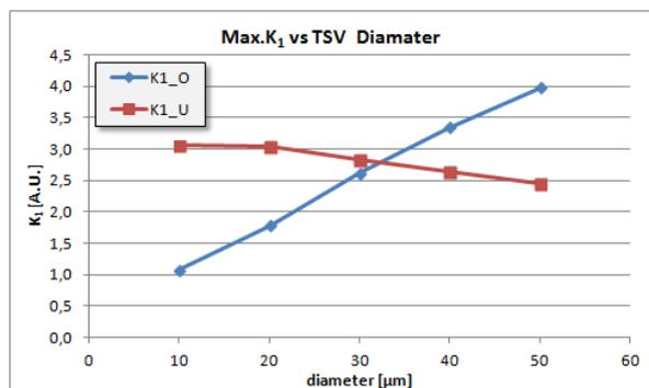
Fig. 9  $K_1$ -progress of both initial material interface crack vs. TSV diameter
