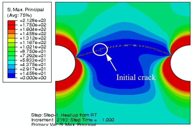
Fig. 13 Initial crack located between the 2 TSVs; heat up from stress free temperature 60 °C to 430 °C
