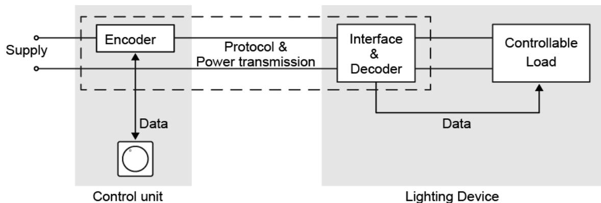
Fig. 1: Block diagram on data transmission of LEDOTRON control unit and lamp
