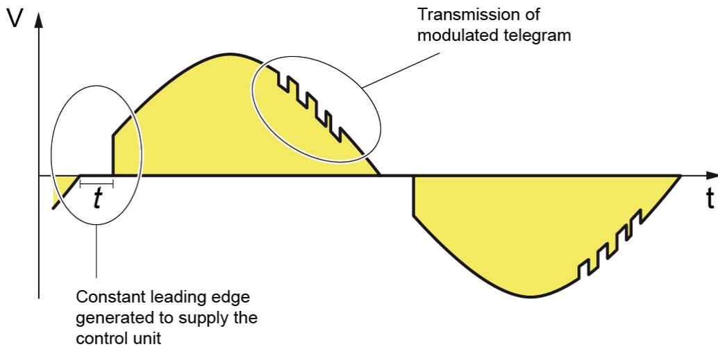
Fig. 2: Signal profile between control unit and lamp
