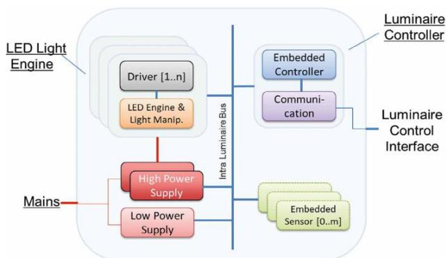
Figure 3: Modular intra-luminaire architecture.
