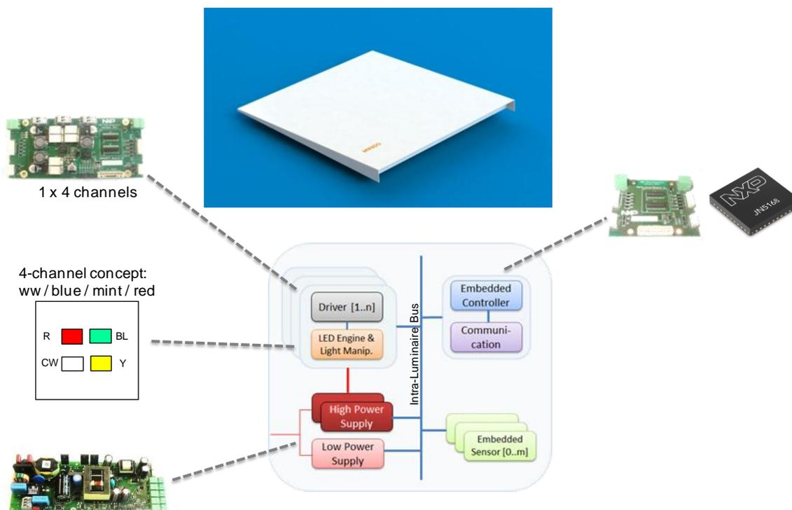
Figure 6: “Wedge” luminaire and luminaire architecture according to Figure 3.
