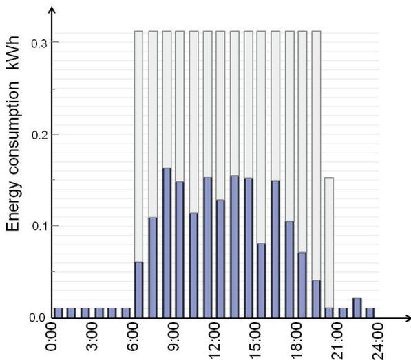
Figure 9: Energy consumption of the lighting installation in the corridor during the course of one day recorded on an hourly basis. Dark bars show the consumption of the EnLight system. Light bars indicate energy
