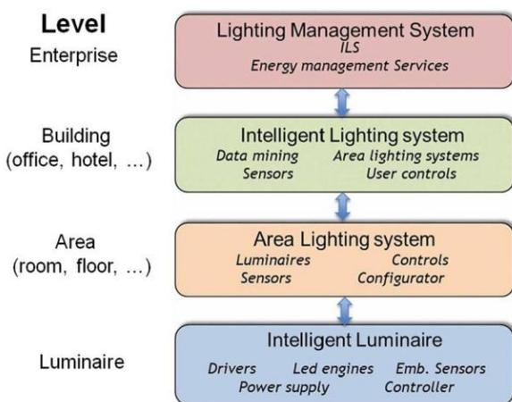
Figure 1: Levels of lighting control. EnLight focus is on “Area” and “Luminaire” level.
