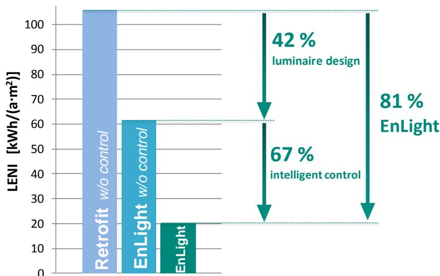
Figure 10: LENI results of the EnLight hospitality pilot installation. For the data without intelligent control, occupancy factors given in [8] are assumed.
