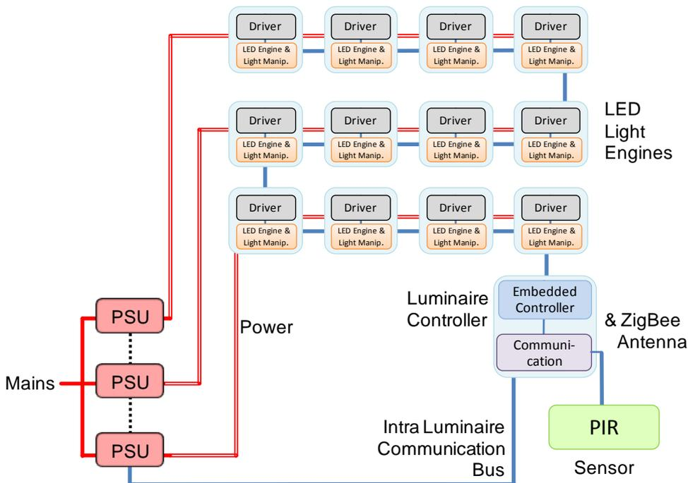
Figure 8: EnLight architecture of the “wedge wall” which can be regarded as one single luminaire. A panel with 12 “wedge” units is shown in this example.
