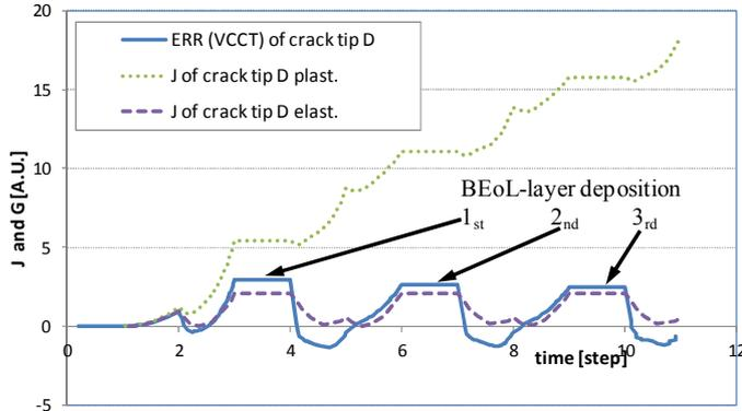
Fig. 2: Jint vs. ERR via VCCT for crack tip D
