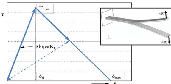
Fig. 3: Traction vs. interface opening in CZM
