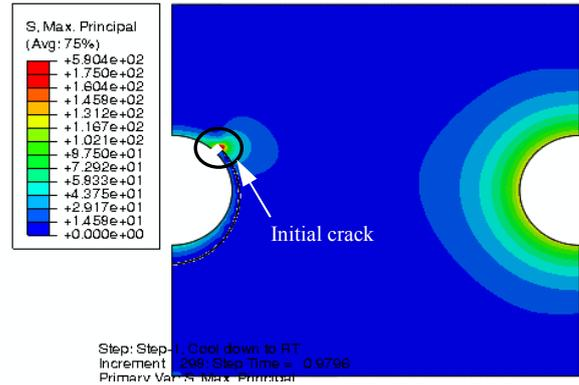
**Fig. 5 Initial crack located at the side wall of one TSV; cool down from stress free temperature 160 °C to RT**
