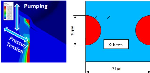
**Fig. 4 Role of CTE-mismatch of Cu-TSVs within Si (left), initial crack located between the 2 TSVs (right)**
