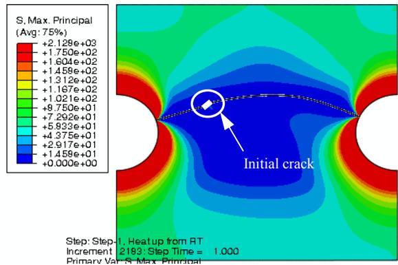
**Fig. 6 Initial crack located between the 2 TSVs; heat up from stress free temperature 60 °C to 430 °C**
