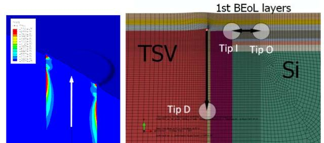
**Fig. 1: Plastic strains in a copper-TSV (left) with existing initial delamination underneath 1<sup>st</sup> BEoL layer (right)**
