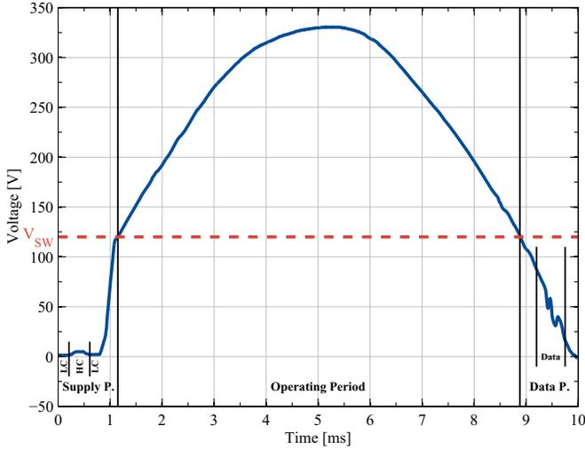
Fig. 2. DLT voltage waveform measured at the input of a 'control gear'.
