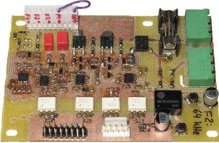
Fig. 11. Photo of the test board including all proposed DLT detector concepts.
