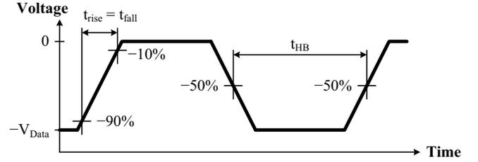
Fig. 3. Specification of physical data transmission.
