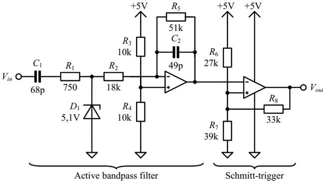
Fig. 6. Schematics of detector #1: Active bandpass with Schmitt-Trigger.
