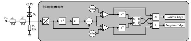
Fig. 9. Schematics of detector #2: Resistive Divider with Digital FIR Filter.
