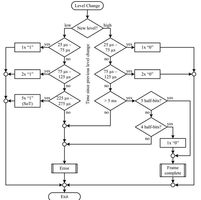
Fig. 7. Flowchart of the implemented DLT frame decoder.
