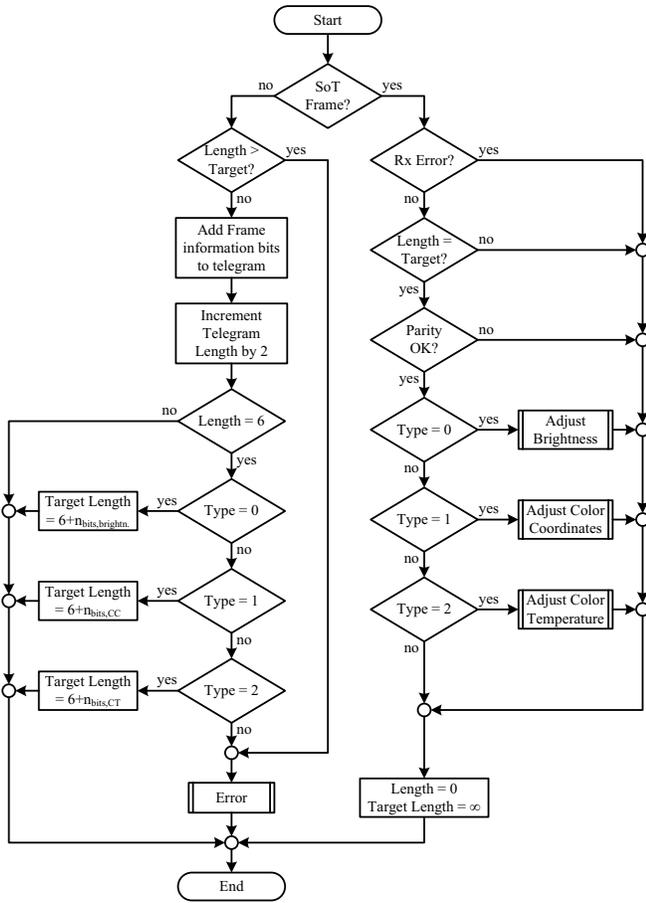
Fig. 8. Flowchart of the DLT telegram reconstruction and evaluation for the most common telegram types.
