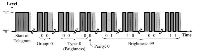
Fig. 4. Example of a single brightness telegram.
