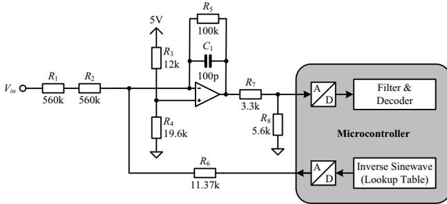
Fig. 10. Schematics of detector #3: Differential analog subtraction filter.
