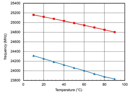
Fig. 10. Comparison of simulated (square) and measured (triangle) oscillation frequency as a function of temperature.
