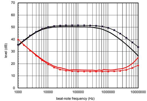
Fig. 11. Comparison between measured and simulated RX noise figure (red, triangle) and conversion gain (black, square). Marked traces represent the simulation results.
