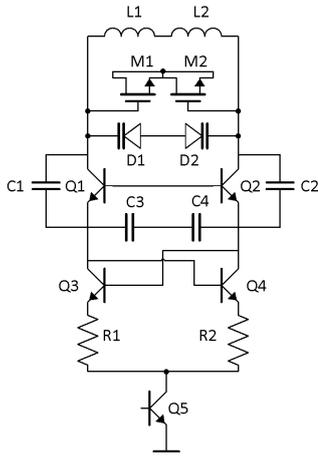
Fig. 2. Schematic of VCO
