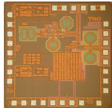
Fig. 3. A microphotograph of the MMIC transceiver (1.1x0.9 mm<sup>2</sup>).
