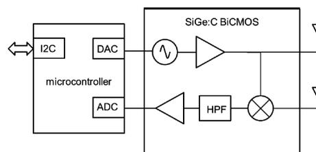
Fig. 1. Block diagram of the FMCW radar system.
